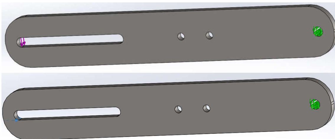
Fig. 7. Simulation loading model of the exoskeleton's thigh link
